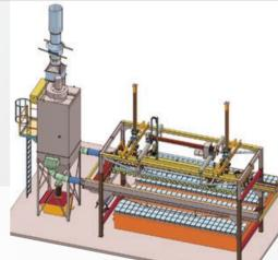
fixed nozzle, the tunnel kiln car runs through a frame from which the suction nozzle specially adapted to the setting plateau is suspended.
